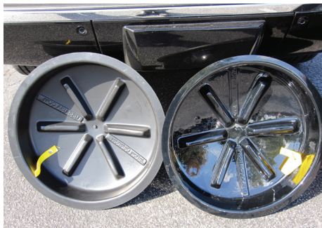
Figure 5. Inflow defender manhole rain dish showing installed dish, and both polycarbonate and polyethylene versions. Note the ribs and depth of dish that improves long-term strength. Note polycarbonate is required for newer, 30- or 48-in. manhole covers. Texas has mandated 30-in. holes for new manholes. Only stainless steel and polycarbonate are available in the larger sizes.
